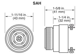
**Mounting Hole:** 1-1/8 in. (29 mm) diameter **Maximum Panel Thickness:** 1/8 in. (3 mm)
